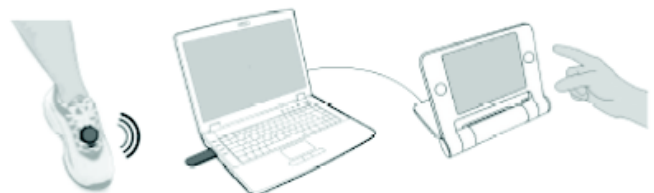
Figure 3. The first prototype consists of three hardware components: a wireless pedometer, a laptop, and a touch-screen.
