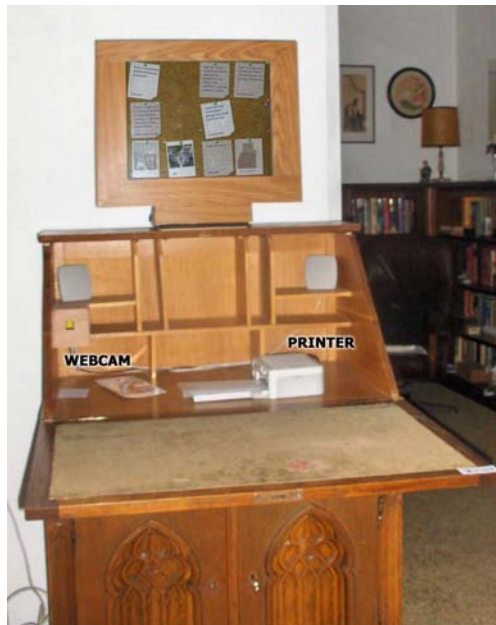
Fig. 5. The final prototype. New messages could be added using a webcam (with the yellow button). Messages could be printed using a printer.
