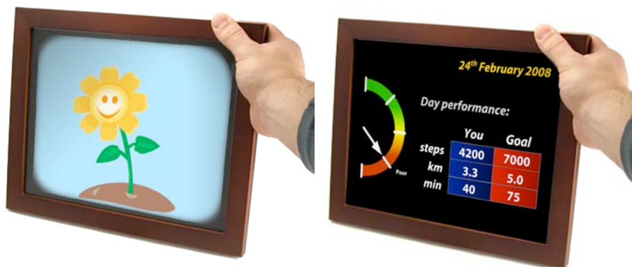
Fig. 2. A photo frame sized touch screen displaying a happy to unhappy flower (left) provides the user with up-to-date information on physical activity. Users can request a detailed overview of the activity levels in respect to preset goals (right).
