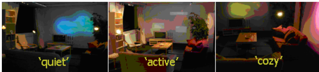
Figure 4. With the prototype atmosphere control system, the ambience of a room (including music, wall art projection and lights) can be changed using a personalized atmosphere model. Left picture: a ‘quiet’ atmosphere, created by a subtly animated blue figure on the wall. Middle picture: an ‘active’ atmosphere, created by bright lights, and moving blocks on the wall. Right: a ‘cozy’ atmosphere, created by warm colored lights, warm colored video art, and use of spotlights
