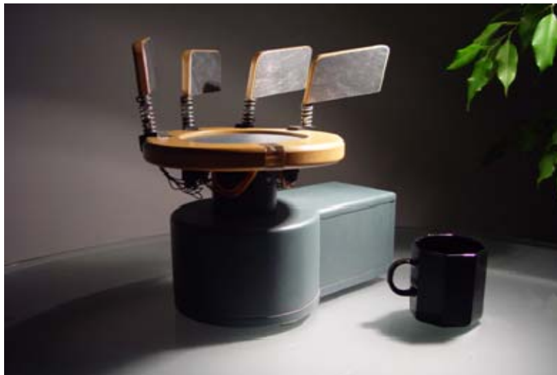
Figure 7. With the Carrousel, a tangible interaction device, users can ‘sculpt’ atmospheres. The stage rotation speed and the orientation of the flags can be changed to express a desired atmosphere
