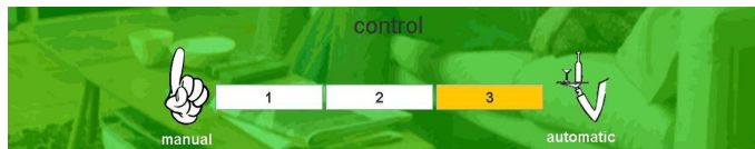
Fig. 1. Using the touch-screen, users could select the preferred level of system autonomy: manual control, semi-automatic, and automatic.
