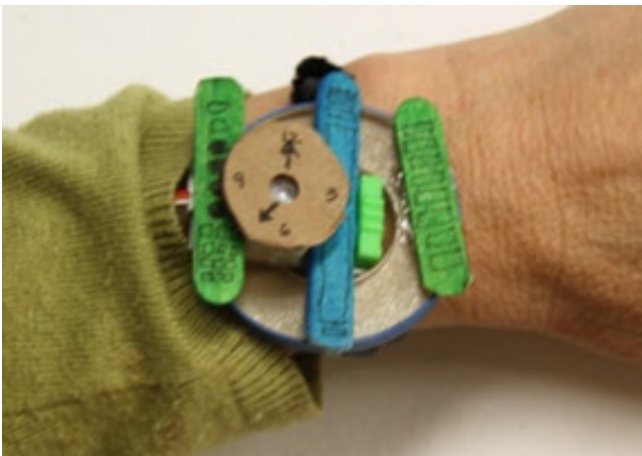
Figure 2. LO-FI cardboard prototype to test layout of physical device
