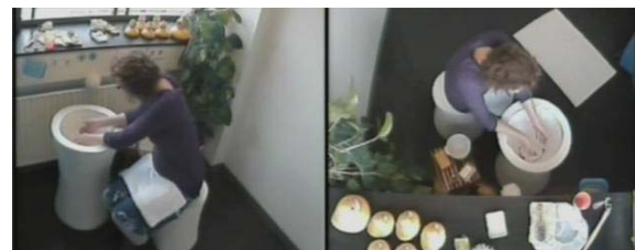
Figure 8: Real size foam model and model with test person in simulated bathroom space
