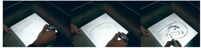
Figure 1: Synthetic Edvard Munch sketches are generated quickly in response to the user's drawing actions. The generated sketches are projected back onto the paper.
