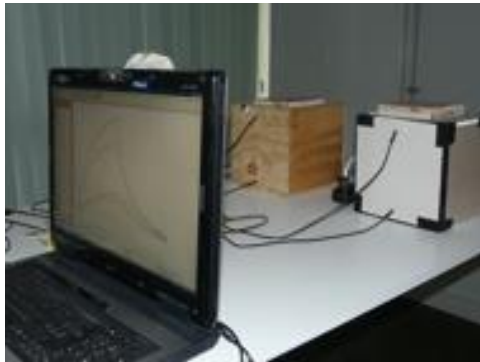
Fig. 5. Two sensors at the same distance from the heater and at the same height from the floor
