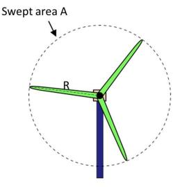
1. Calculate the output power in Watts from a wind turbine which has a rotor blade radius of 6 metres with an efficiency of 40% in an area where the air density is 1.225Kg/m3 and where there is a wind speed of 8 m/s. Show your work below...
