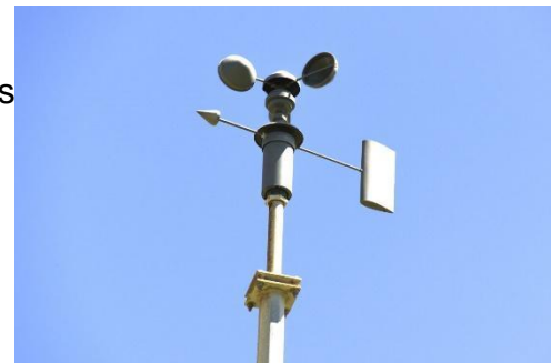
Figure 1: Anemometer and wind vane up close
