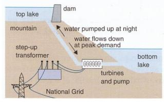
The water cycle (rain) can be used to fill up reservoirs. The water is allowed to fall from the dam through a pipe. This fast-flowing water is used to turn a turbine, which spins and drives a generator. The generator generates electricity.
