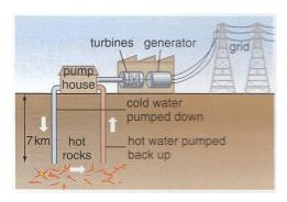
Geothermal (Geo - Earth, Thermal - heat) power stations use heat from the hot rocks deep inside the Earth. Cold water is passed down a pipe to the rocks. The water is heated by these rocks and turns into steam. This steam is then used to turn a turbine.
