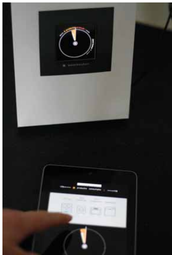
figure 3.18c Two tablets appear as wall mounted (on top) and a single tablet is available for portable wireless use (bottom). The wall mounted tablets form the 'integration-layer 1', of the concept and are not recognisable as tablets, they seem integrated with the Niko Home Control system, which is present in the house. The wireless portable tablet runs the 'learning-layer 2' application which allows people to get detailed insights in their electricity status and use.
