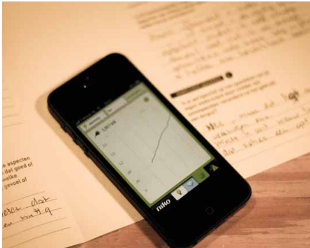
figure 3.24 An example of the interface in situation 'A', of the Niko Home Control system. The screen which tells the user the most is where the net-total is presented, this subtracts the production from the total consumption.
