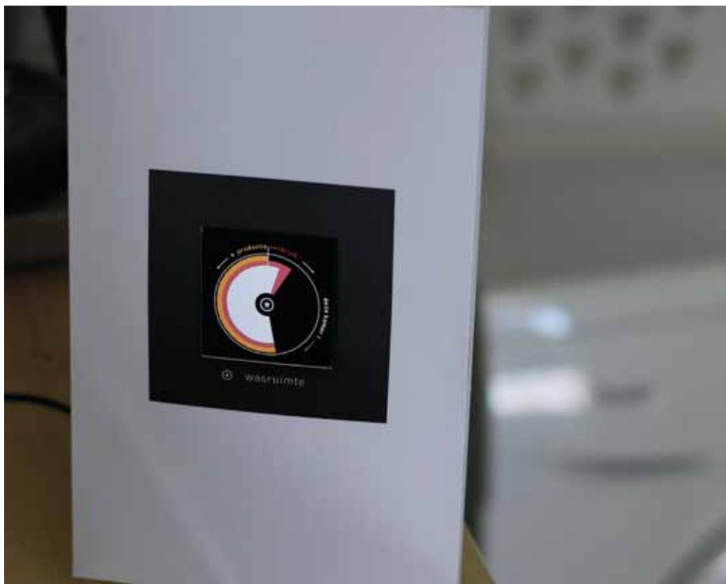
figure 3.26 The prototype featured part of the total design, which enabled users to monitor their current electricity consumption and production (prosumption) in real time. In this figure is visible how the heating element of the washing machine is working. In a glance can be understood that this is almost done with solely solar energy.
