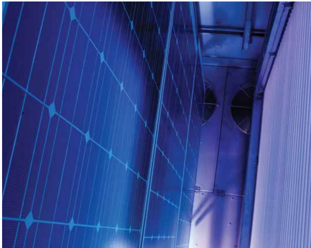
Figure 1.10 A special climate chamber with UV light for the artificial aging of photovoltaic modules in TÜV Rheinland's solar laboratory.
