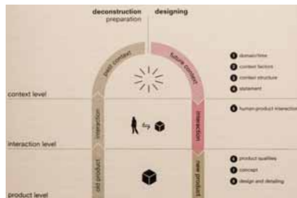
figure 3.3 8 steps of the ViP method which will be part of the process, step 1 to 3 will be used to define a context from the relevant factors which have been discovered during the (user) studies.
