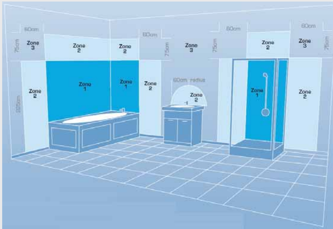
Figure 14: Bathroom Electrical zoning illustration
