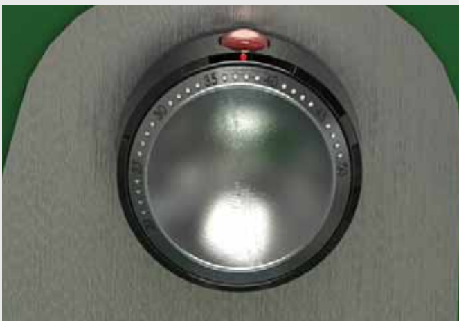
Figure 73: Close-up of safety faucet control
