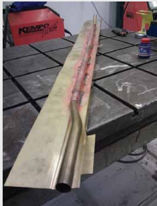
Figure 61: Soldering the radiator
