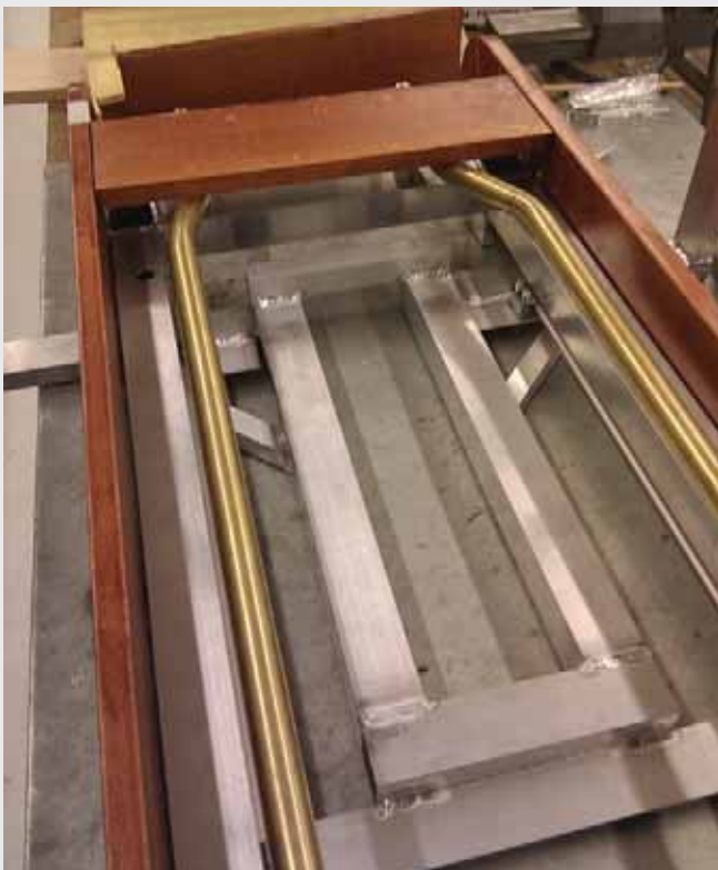
Figure 47: Brass piping mockup
