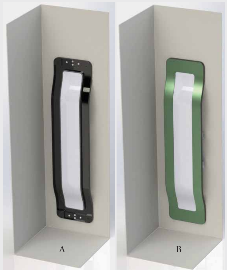
Figure 68: Console with mirror installed (a) and with radiator panel installed (b)
