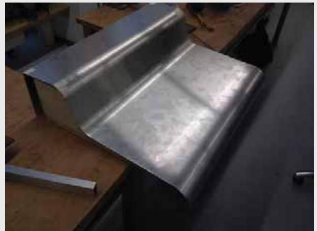
Figure 46: Worktop panel fabrication
