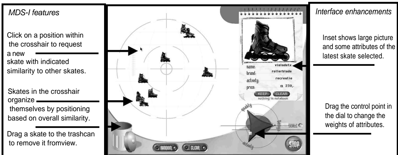
Figure 1. An MDS-Interactive interface to a database of skates (graphic design: Bram v.d. Nouweland).
