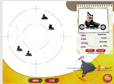
Figure 6.8 The selection triangle (bottom right) can be used to increase the weight given to either quality, design or activity. By moving the selection slider to the lower right-hand point of the triangle, the user gives more value to "activity" in the MDS procedure. This causes skates, which are suited for a similar activity, to be grouped closer together, and further away from the other types.
