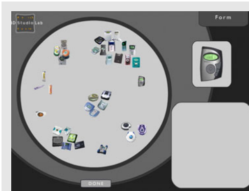
Figure 6.17 By putting samples into the interaction circle, mutual relationships between them are being established, without having to attach keywords to each sample separately. When the designer is satisfied with his arrangement, clicking the "Done" button the system calculates and stores the distance between each pair of samples.
