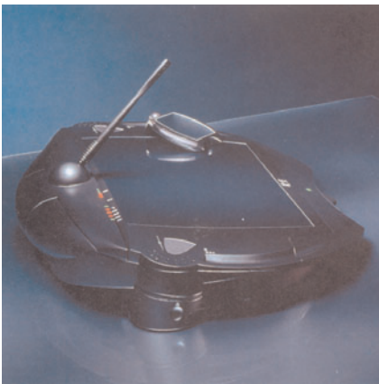
Figure 2.24 Time, a two- handed sketching device
