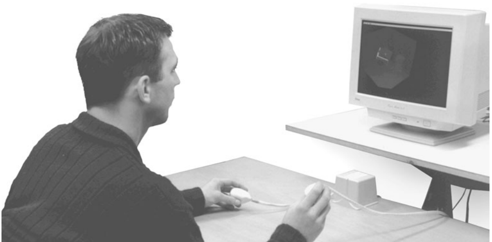
Figure 2.23 Two-handed interaction using the Frog input devices.
