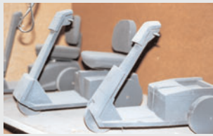
Figure 2.2 Simple mock-ups out of foam are quickly created to explore features that are difficult to evaluate in two dimensions, such as volume proportions.
