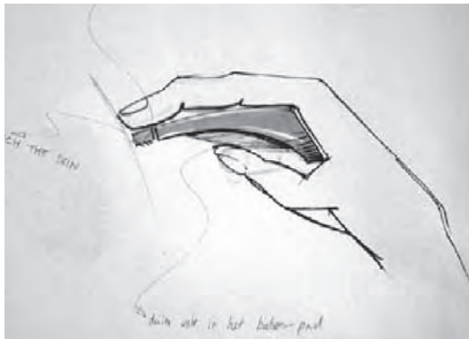
Figure 5.1.2 One of the concepts generated by the designers in the evaluation: A razor held inside the hand, establishing continuous contact between the skin of fingers and face.
