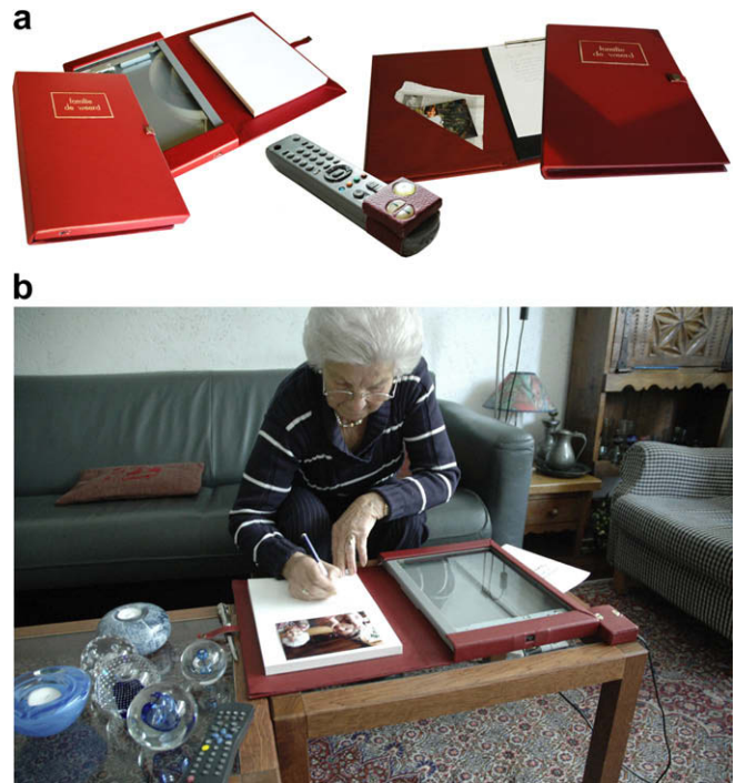
Fig. 9. The working prototype consists of a notebook with a scanner in its cover, and a small extension to the television's remote control.
