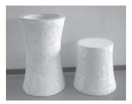
Figure 7-18 Foam prototype of the first splash design.
