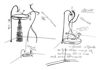
Figure 3 Sketches of the '1Sink' concept
