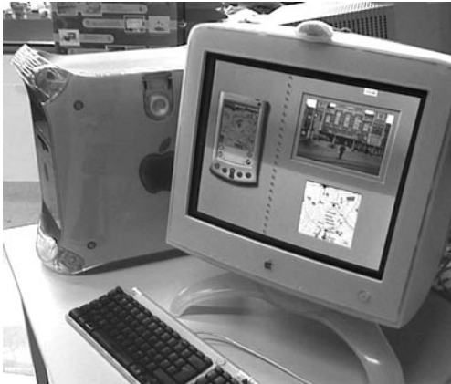
11 Screen-based setup for testing handheld navigation interface
