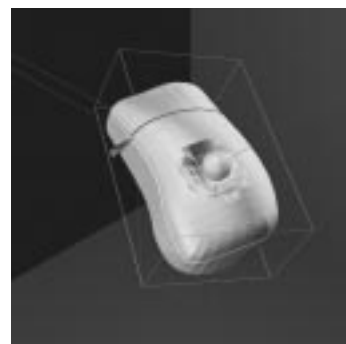
Figure 3-32. The state of the model after activation of the sculpt tool. The right hand has moved the sphere into the surface, thereby displacing vertices.
