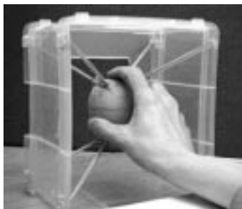
Figure 2-12. The EGG, an elastic sensing device.
