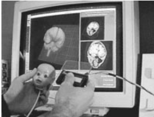
Figure 1-18. Two-handed 3D input with props devices.
