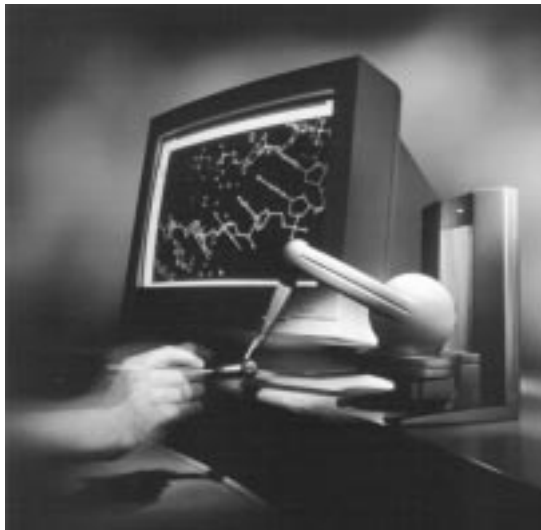
Figure 1-14. The Phantom interaction device with haptic feedback.
