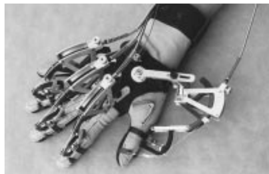
Figure 1-15. The CyberGrasp glove with haptic feedback.
