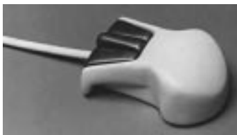
Figure 1-10. The 6D Mouse of which both position and orientation are sensed.
